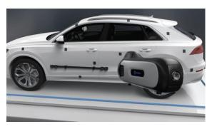
Place the coded targets and scale bars and take photos from different angles and positions. Photos taken show up in Glopho in real time.
