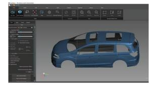
Generate highly accurate 3D modes which can be compared with original CAD models to generate intuitive reports or serve as a data basis for further design.
